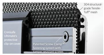
All Crimsafe products feature our patented Crimsafe Screw-Clamp™ technology. Tamper resistant screws first go through a metal clamp, then through Crimsafe's Tensile-Tuff® mesh and then driven right into the frame, to hold the mesh in a "vice like" grip. This patented Screw-Clamp® gives Crimsafe screens enormous strength against attack, unlike inferior products that simply glue or wedge mesh into a frame.
